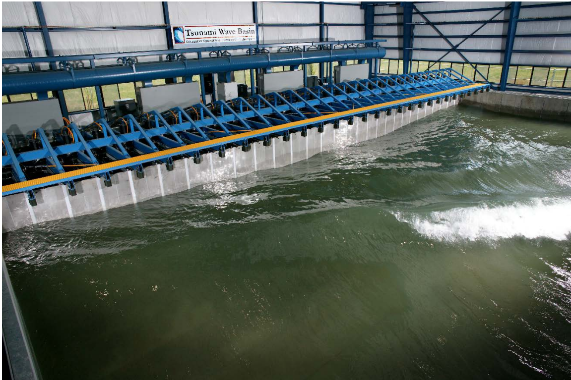
Figure 2. Wave maker of the Directional Wave Basin.
