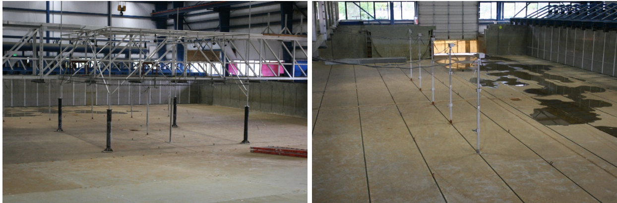
Figure 5. Instrumentation deployment in the DWB. Left, motion tracking frame and nominal model location. Right: wave gauge array for “far-field” wave conditions.
