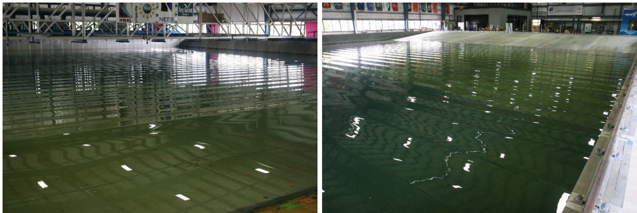
Figure 6. Wave calibration testing.
